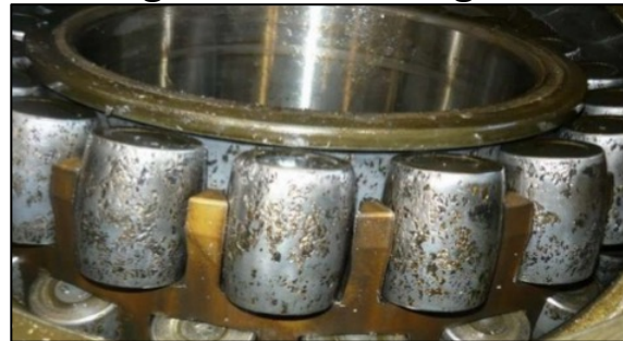
Rolling element damage
