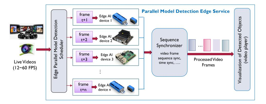
Single Edge node attached with multiple Al-hardware devices, each runs one detection model
